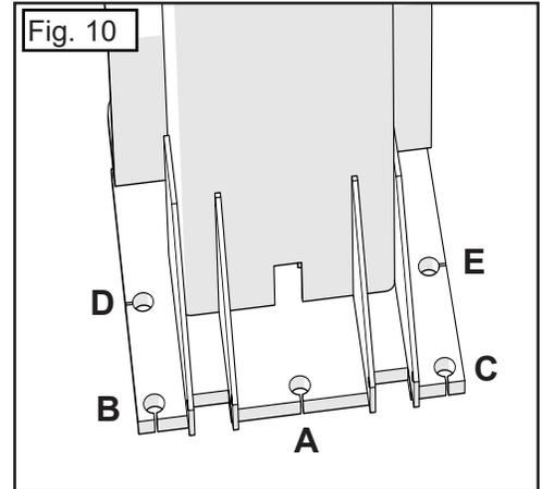
**NOTE:** The drill will break through the bottom when drilling 5" in a 4.25" concrete slab. This is an approved practice with these Anchors.
