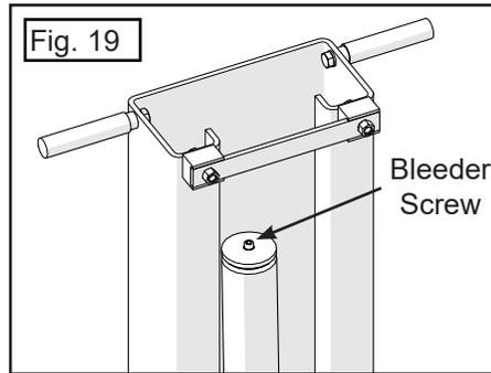
6. With no weight on the Lift, raise the Lift to its maximum height and check the Bleeder Screws for air bubbles or oil escaping as the Lift is rising. Air will continue to exist from the loosened bleeder screws.
