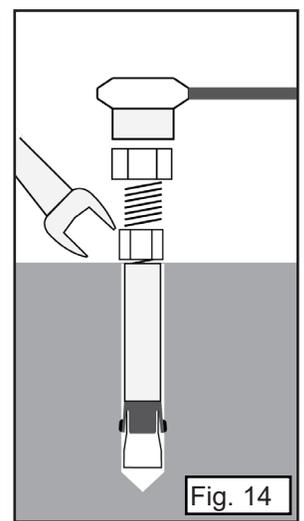
7. Install both Posts with Bolts and Washers to Anchors, check plumb and measurements as shown below.
