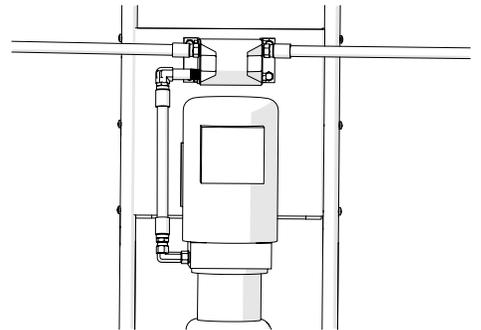
If your Flow Divider looks like the graphic below, **rotate the Flow Divider 180°** so that the side with an **IN** and **OUT** Port is on the **right** side, and then connect the Short Hydraulic Hose to the Lower **IN** Port; the other end of the Short Hose connects to the Pressure Port on the right side of the Power Unit..
