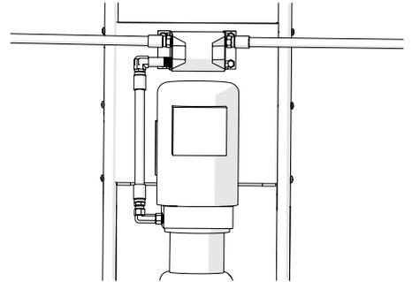
If your Flow Divider looks like the graphic below, the Left side Ports are **mislabeled**. **Do not connect the Short Hydraulic Hoses to the Top Left Port**. Connect the Short Hydraulic Hose connects to the Bottom Left Port, and two Long Hydraulic Hoses connect to the Top Ports on either side of the Flow Divider.
