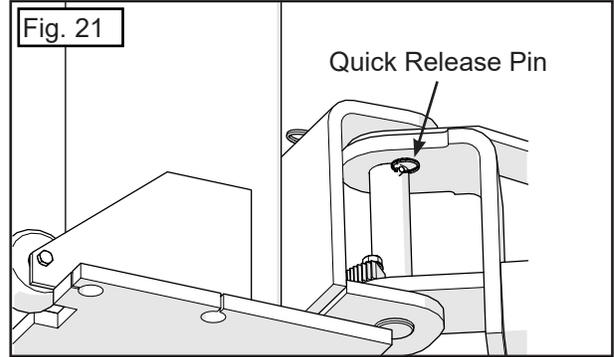
2. Raise the Lift high enough so that the Arm Gear stops. Attempt to automatically engage the Restraint Gears on the Arms.
